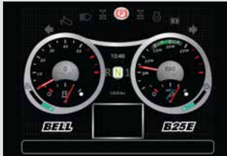
A user friendly 10" colour monitor offers vital operating information, safety warnings, detailed diagnostic readings and dump body function settings.
