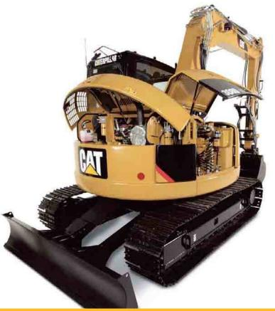
Robust, reliable and easily serviced are the key attributes of Caterpillar Mini Hydraulic Excavators. Full steel body work panels provide durable protection against damage. All daily service points are easily accessed through the rear hood and side cover and a 500 hour engine oil change interval lowers operating costs. The Cat S•O•S. points assist easy oil sampling for preventative maintenance checks.
