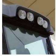
4 front working lights and 4 rear working lights (on all models equipped with variable flow pump)
