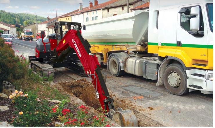
The vio80-1 offers the performance of a large excavator while enjoying the benefits of a compact excavator. Particularly suited for work in urban areas, it can operate with confidence and efficiency along the walls and in confined spaces where the machines in its weight class do not have access.
