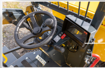
Protected IP67 rated 7" LCD Monitor
