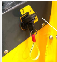
Two stage start inhibitor safety system
