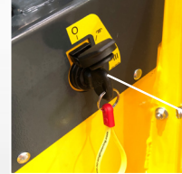
Two stage start inhibitor safety system
