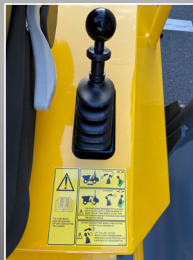
Hydraulic parking brake (SAHR) No in field adjustment required
